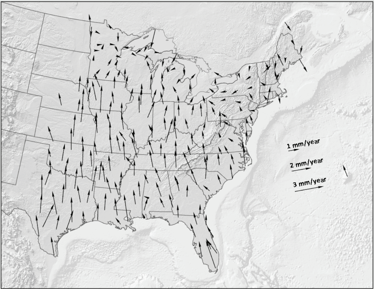
Figure 2: Horizontal non-Eulerian velocities (observed minus Euler-derived) to the east of longitude 250°. Their magnitude is smaller than 2 mm/year. It is expected that those stations which were used to derive the Euler pole will behave well (have small non-Eulerian velocities) while other stations may have larger non-Eulerian velocities.
