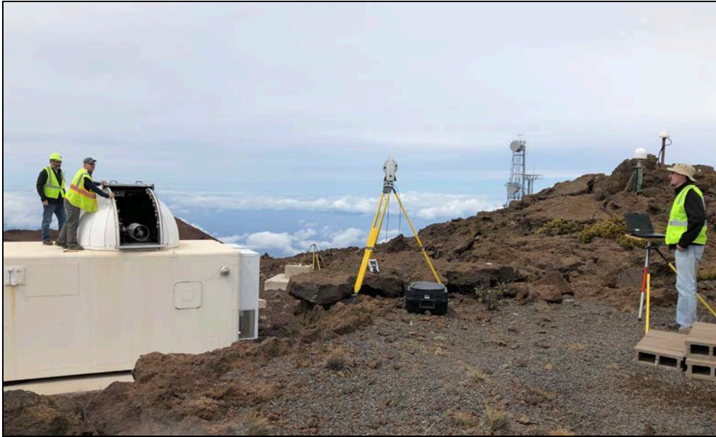
Target/reflector affixed to SLR antenna for azimuth and elevation rotation sequences
