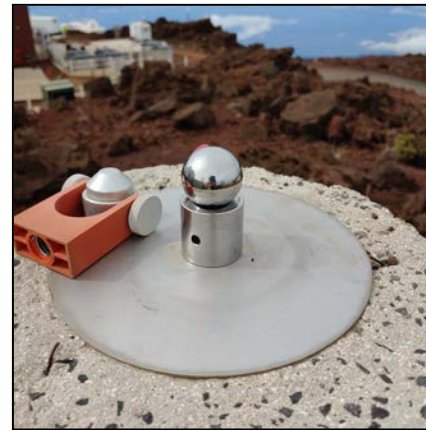
Reflector occupying CAL PIER A
