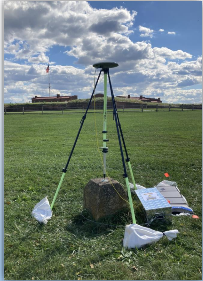
GNSS Occupation on 84TB adjacent to Fort McHenry - Oct. 2021 (Photo Credit: Heather Quinn – MGS)
