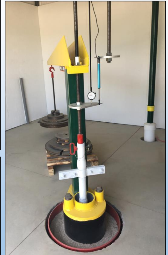
Pictured: Nansemond Extensometer at HRSD's Sustainable Water Initiative for Tomorrow (SWIFT). Source: USGS, Public Domain
