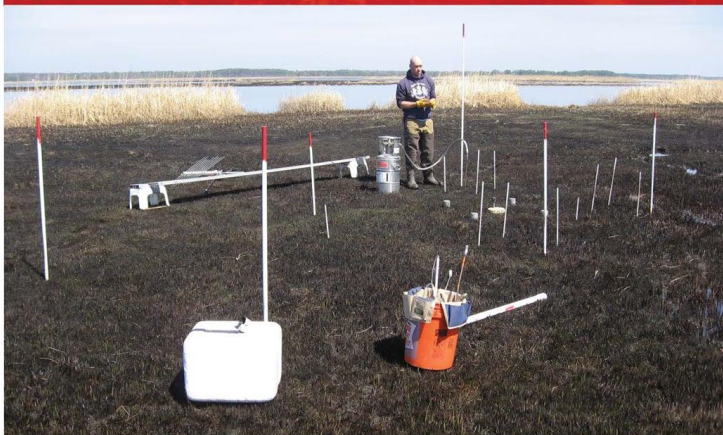
A burned marsh plot in Blackwater National Wildlife Refuge, Maryland, with equipment for collecting an accretion core from a marker horizon.
