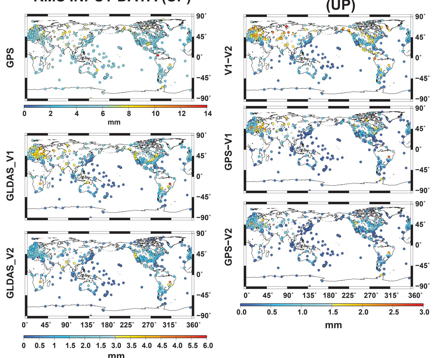
V1 is more variable over Europe than V2. V1 does better at removing signal over Europe and North America as compared to V2.
