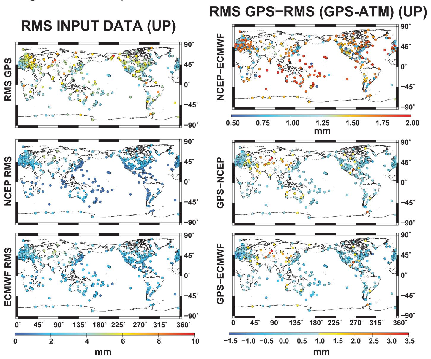
Of the 514 stations with more than 100 weeks of observations: GPS - NCEP: 406 of 514 station RMS improved; GPS - ECMWF: 282 of 514 station **RMS** improved Results appear to indicate that NCEP fits the GPS residualsbetter than the ECMWF
