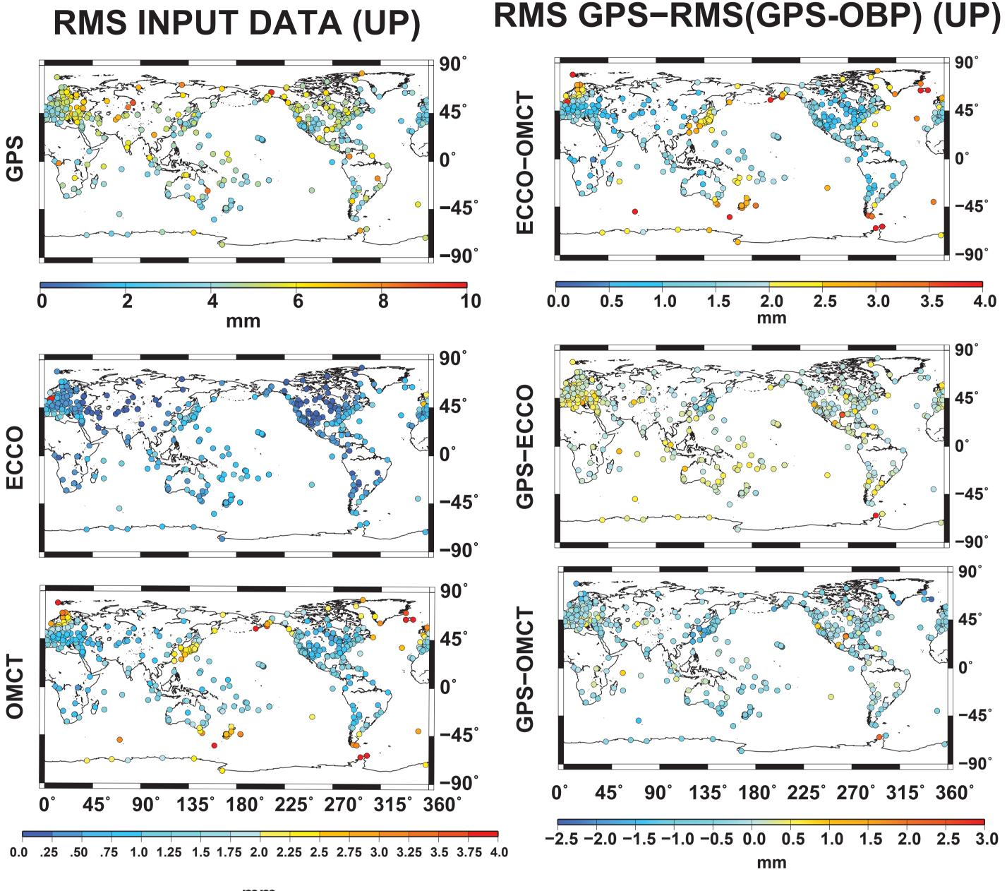
Of the 514 stations in this data set, ECCO reduces the RMS on 407 while OMCT reduces the RMS on only 85. These results indicate that the ECCO model is more valid at longer wavelengths and at periods > weekly as compared to OMCT.
