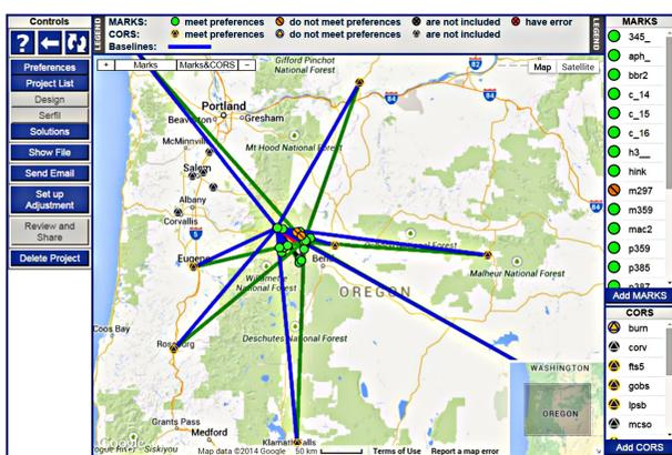
**Figure 7.** OPUS-Projects manager's page with project map, indicating project CORS and user marks, processed project baselines, and various software navigation controls.
