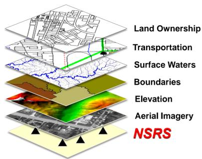
**Figure 1.** Typical geospatial data layers and NSRS, the foundation layer which provides a common spatial coordinate system and allows data from disparate sources to be attributed and analyzed within a consistent spatial framework.
