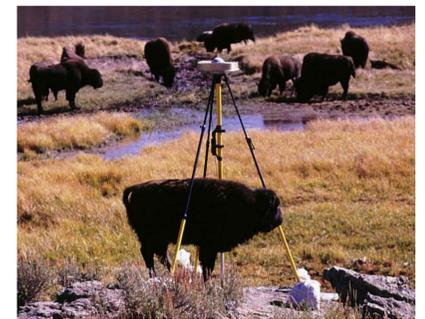
**Figure 2.** GNSS survey occupation for geophysical research and curious bison in Yellowstone National Park, Wyoming, USA. CORS and OPUS greatly simplify field logistics for precise positioning in geospatial projects.
