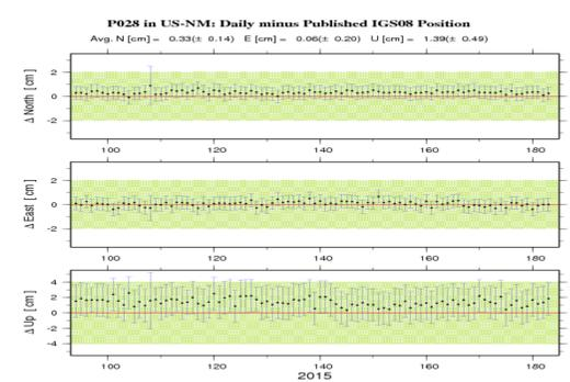
**Figure 4.** 90-day repeatability plots and summary statistics of CORS site P028 daily station coordinates (north, east, up) minus published IGS08 coordinates. Green shading indicates standard CORS positional tolerances; error bars are 1-sigma. Similar plots are generated daily for all CORS to monitor station and network consistency and reliability.
