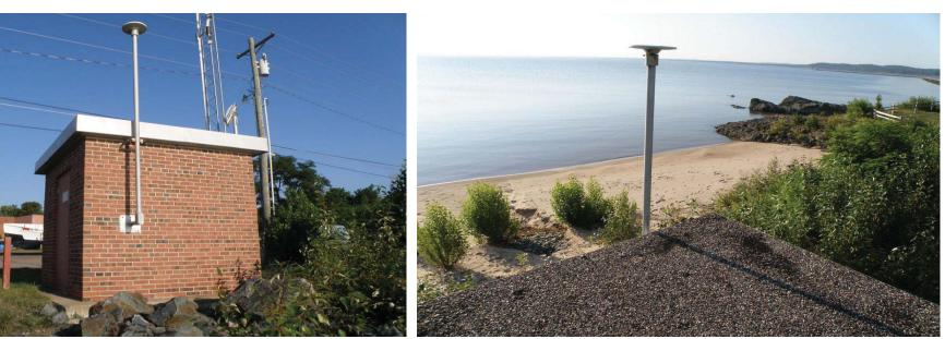
Figure 3. WLS and collocated CORS i(MIMO) n Marguette, Wisconsin. Distance was measured from CORS ARP to the Eletronic Tape Gauge (ETG) on the bench in the structure. Drops are made from the ETG table to a well freely connected to the water surface. When the sensor hits the water and completes an electric circuit, the distance is recorded. This provides a means to transfer the water level surface into geometric coordinates.
