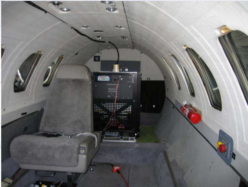
The NGS airborne gravimeter (“TAGS”) mounted in the NOAA Cessna Citation and ready for flight
