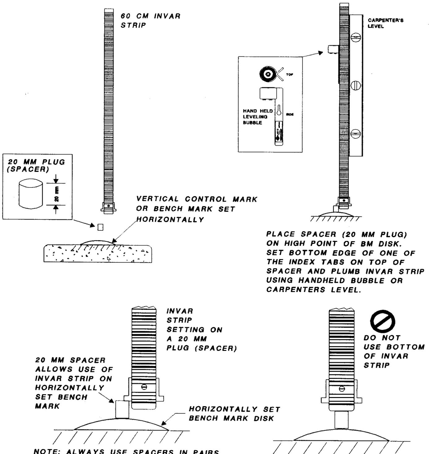
**NOTE: ALWAYS USE SPACERS IN PAIRS ONE AS SHOWN ABOVE AND ONE ON THE BACKSIGHT ROD. IF YOU ONLY HAVE ONE SPACER, PUT IT ON THE BACKSIGHT AND READ IT. THEN PUT IT ON THE FORESIGHT AND READ IT.**
