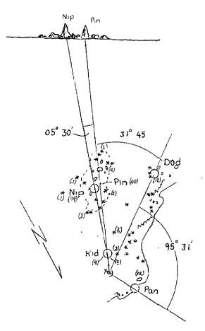
Sextant angles taken from anchored launch. Three point fix with check angle plotted on vinylite copy of map manuscript. Distance from launch position to NIP scaled. Vertical angle to top of pinnacle (NIP) read on and off the sextant circle.
