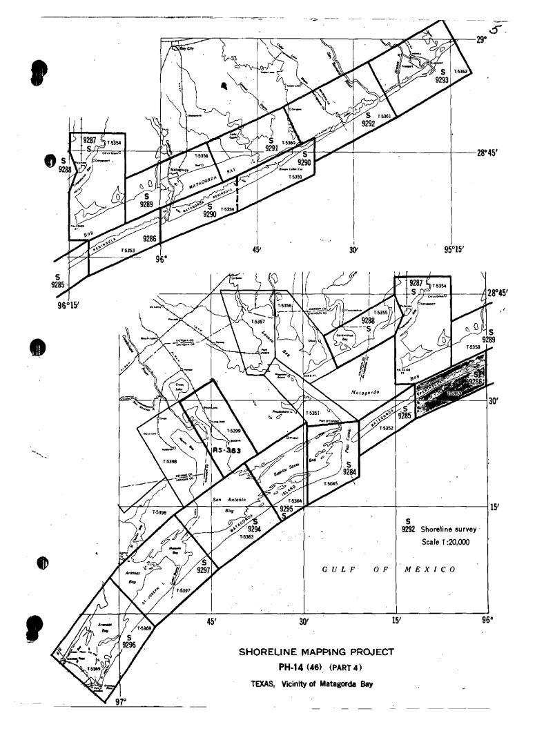
Shoreline survey T-9286, scale 1:20,000, (Latitude 28° 30' to 36'; Longitude 96° 00' to 12'), is one of 76 maps in project Ph-14(46), Intracoastal Waterway, which consists of four parts.
