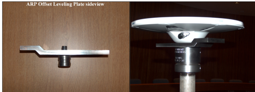
Figure 1. Left image: An offset leveling plate.
