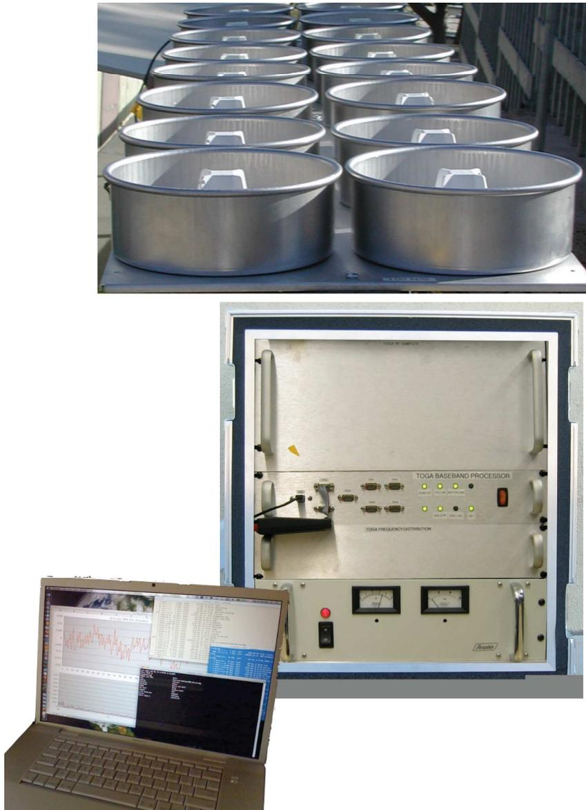
FIGURE 10. JPL's TOGA (Time-shifted, Orthometric, GNSS Array) instrument.
