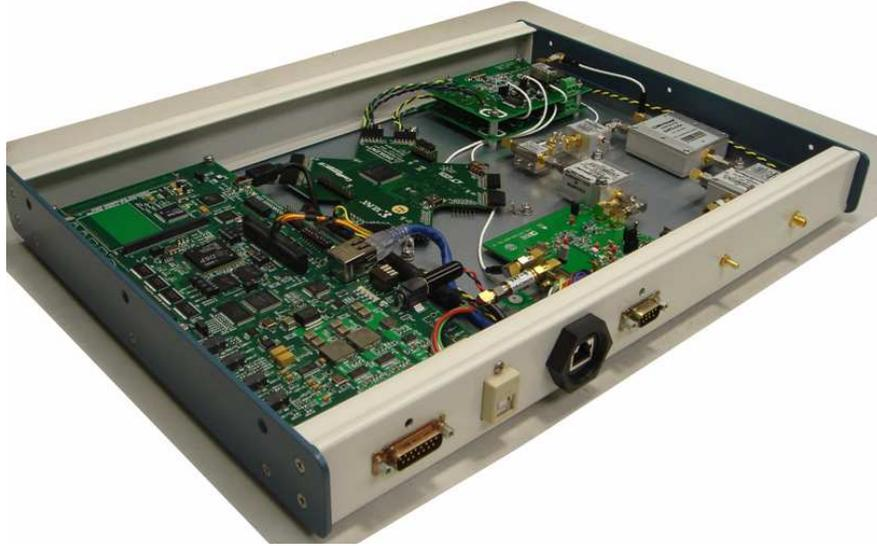
FIGURE 8. The Cornell University GRID (GNSS Receiver Implementation on a DSP) instrument.
