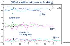
processed passes on a GPS satellite, initialisation step (stations clocks are defined, estimation of consistent ambiguities and satellite clock)
