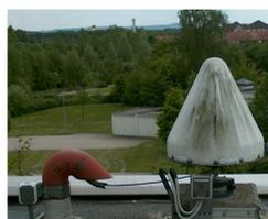
Reference station 1000 with reflectors in the near-field
