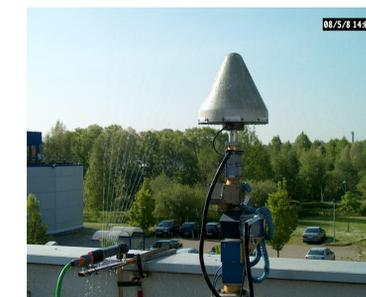
Sprinkling of chokering antenna with SNOW radome during antenna calibration
