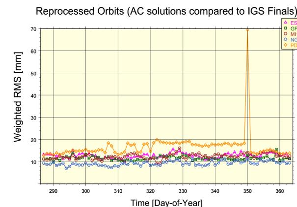
Fig. 3. Eleven weeks of weighted 1D RMSes from reprocessed orbits compared to IGS Final orbits.
