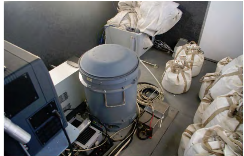
Relative gravimeter Chekan in a cabin of AU
