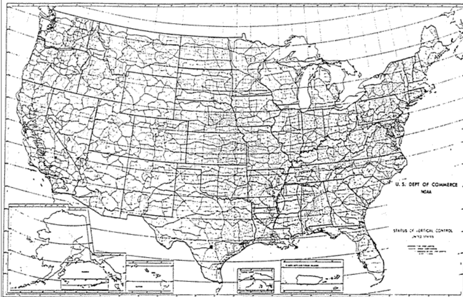
Figure 3. Vertical control used in 1988 adjustment.
