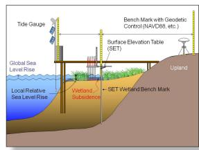
Connecting tide gauges and SETs to an accurate vertical datum is essential for coastal sea level-change monitoring and risk assessment.
