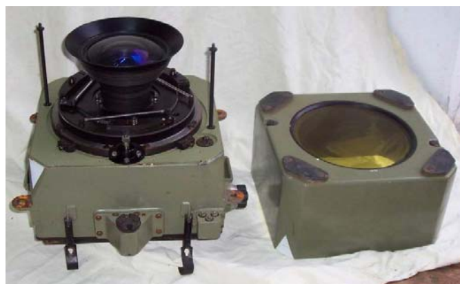
A Wild Co. RC-5a camera with filter cowl removed
