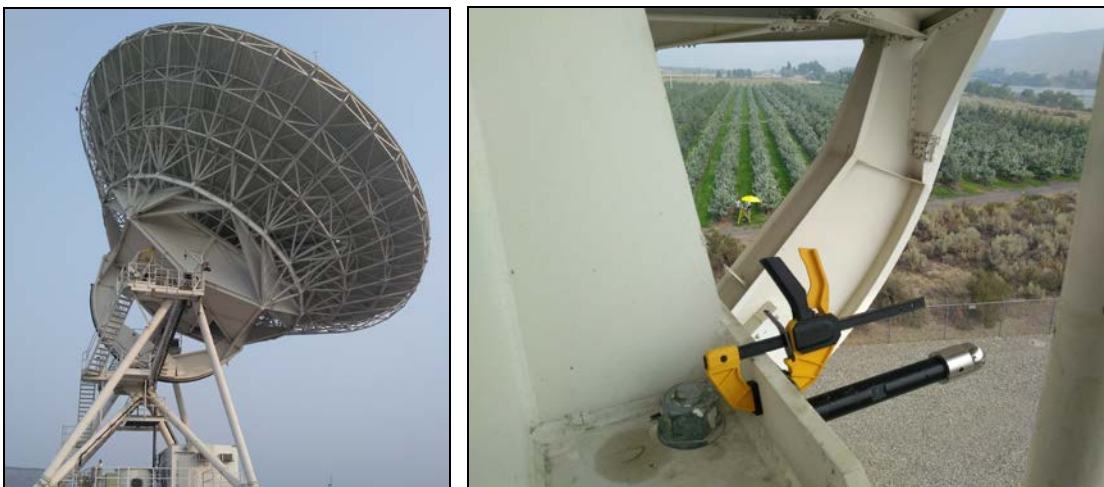
Figures 9, 10 – Target/reflector affixed to VLBI antenna for azimuth and elevation rotation sequences
