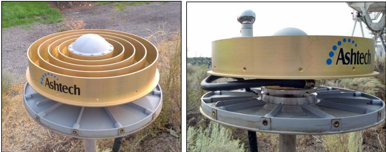
Figures 11, 12 - Observations of the choke ring were used to determine GNSS reference point through circle-fitting
