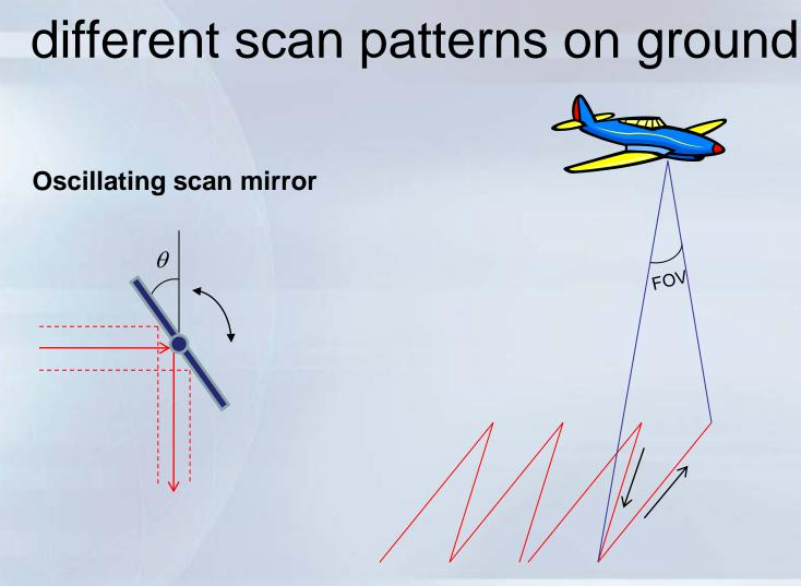
Different scan mechanisms =>
