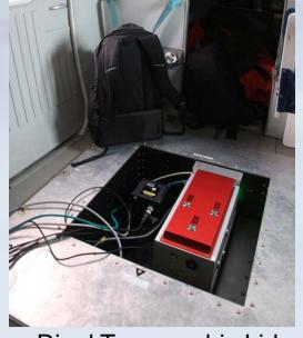
Riegl Topographic Lidar (LMS-Q680)
