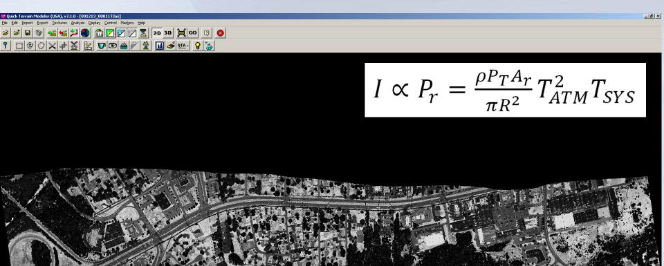
Point cloud color-coded by intensity in QT Modeler
