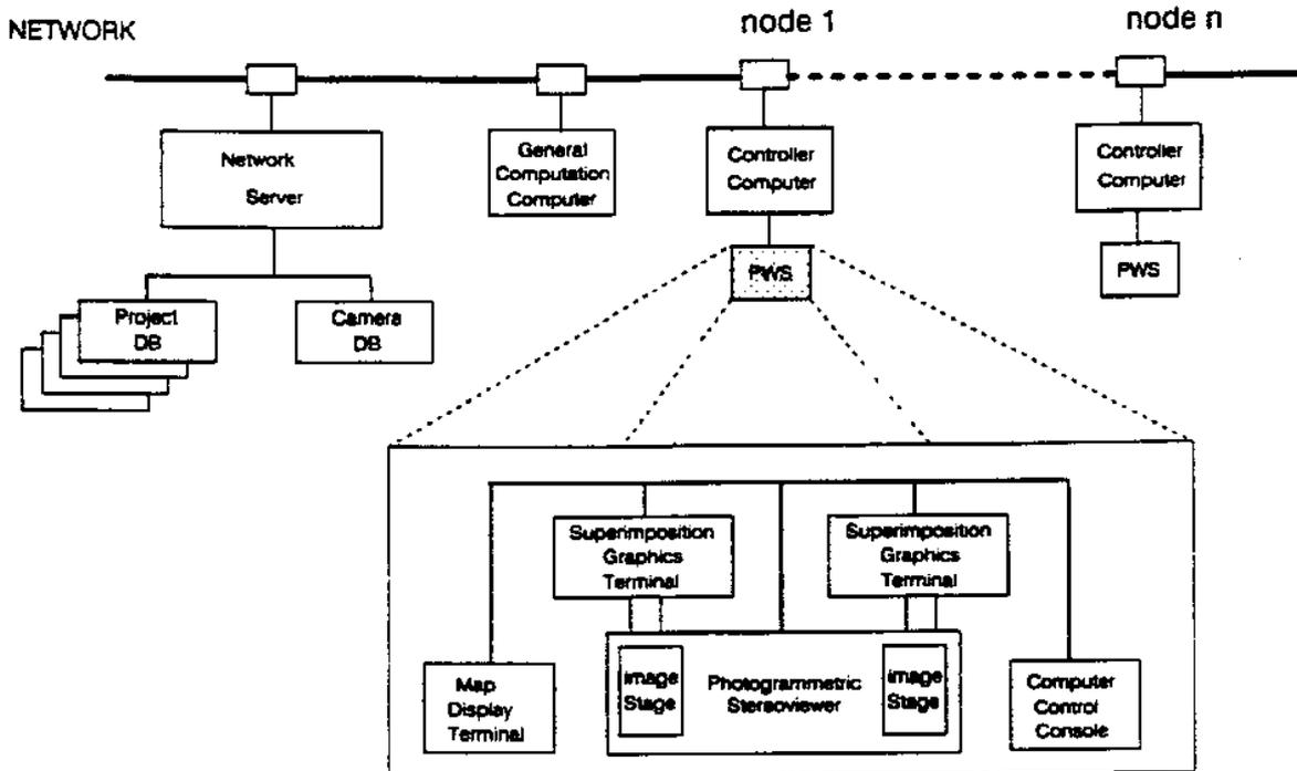
Figure 3.--IDPF system architecture.
