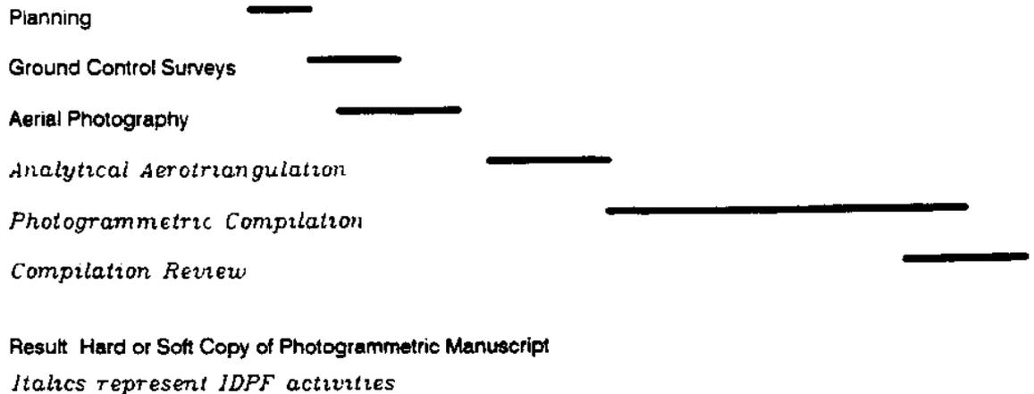
Figure 2.--Stages of a photogrammetric project.
