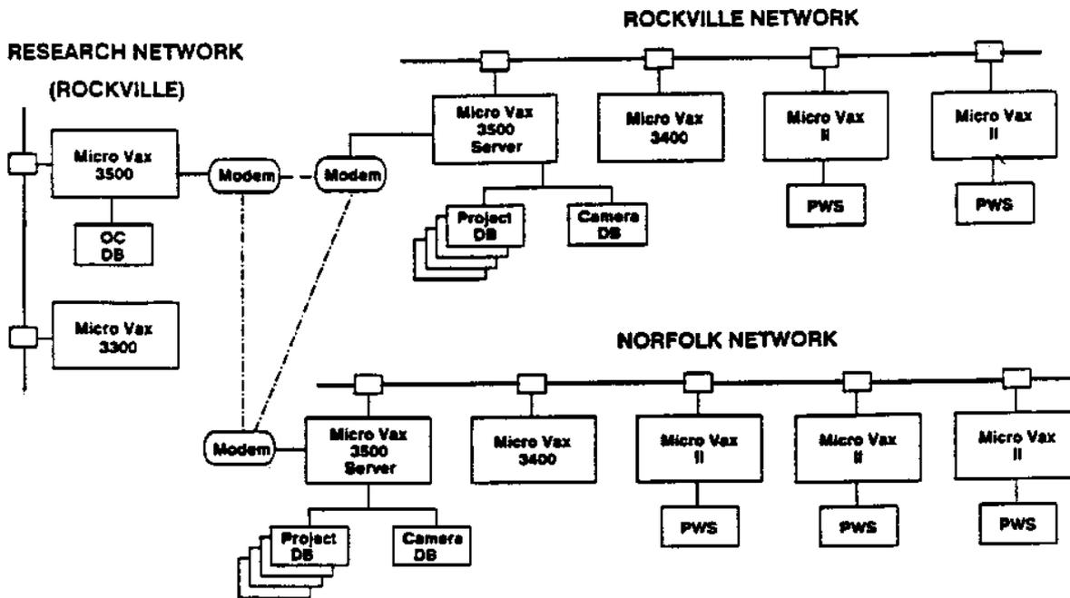
Figure 1.--IDPF system configuration.
