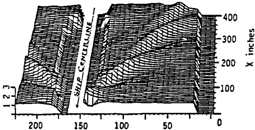
Figure 7.--Photogrammetrically derived wave heights.
