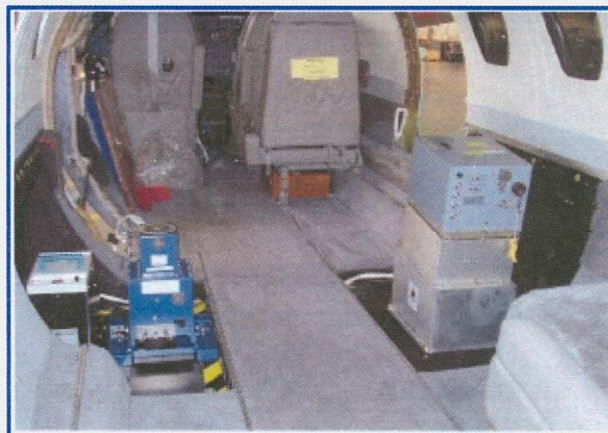
Figure 2: The Itres CASI-2 hyperspectral imager, Emergel/Applanix Digital Sensor System (DSS), and an Optech ALTM 2050 system installed on the NOAA citation aircraft (left to right). Click on image to see enlarged.
