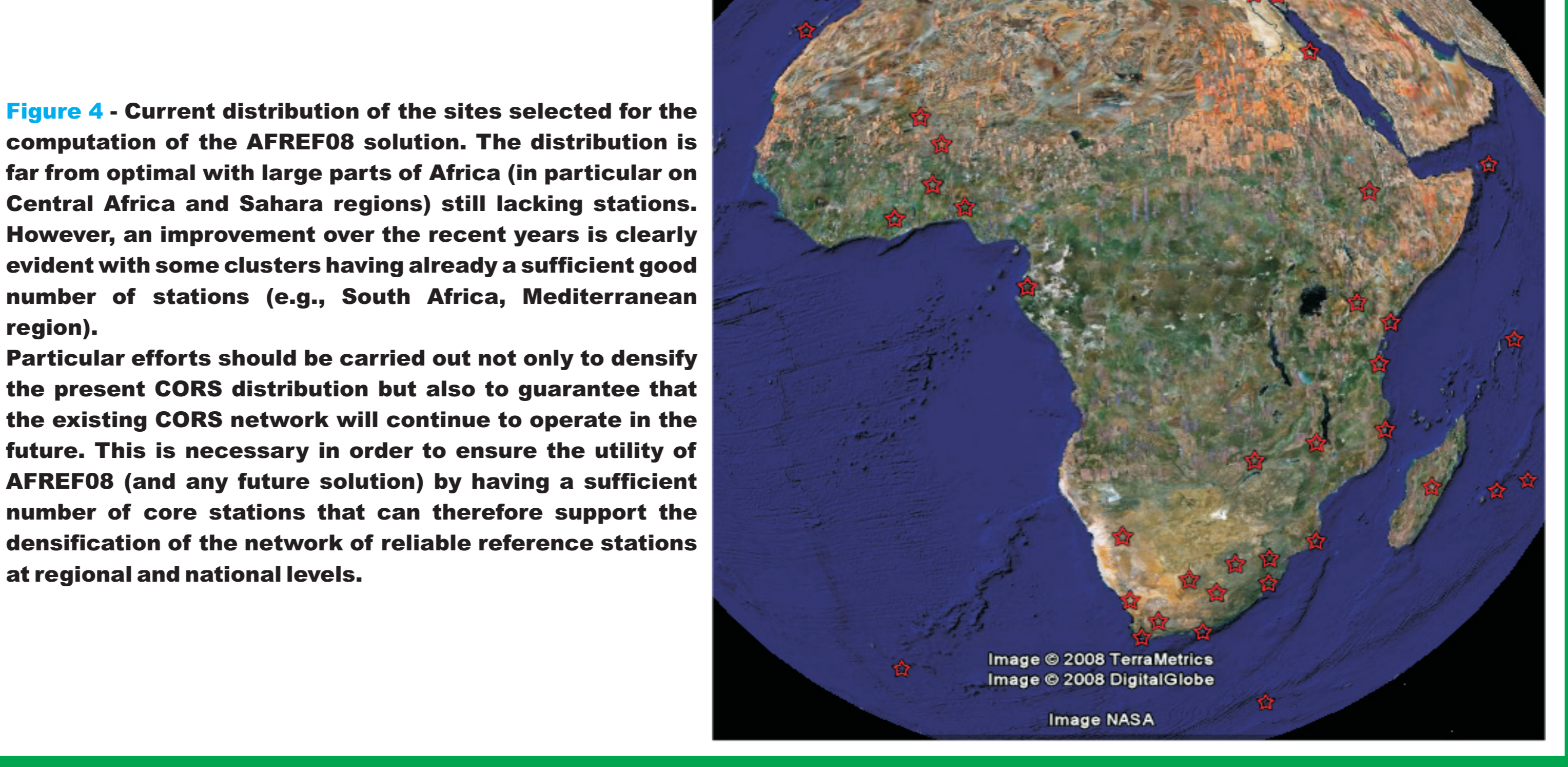
Figure 3 - (Left) Distribution of the CORS IGS network in the African continent; (Right) IGS Stations included in the computation of the AFREF08 solution. Out of 21 individual stations that are officially part of the IGS network in the African continent, only 13 sites could be selected. Eight stations were not operational during the period of interest. The situation is more critical on West Africa where all three stations integrated in the IGS network (Cape Verde, Senegal and Côte d'Ivoire) are not operating for a long period of time.
