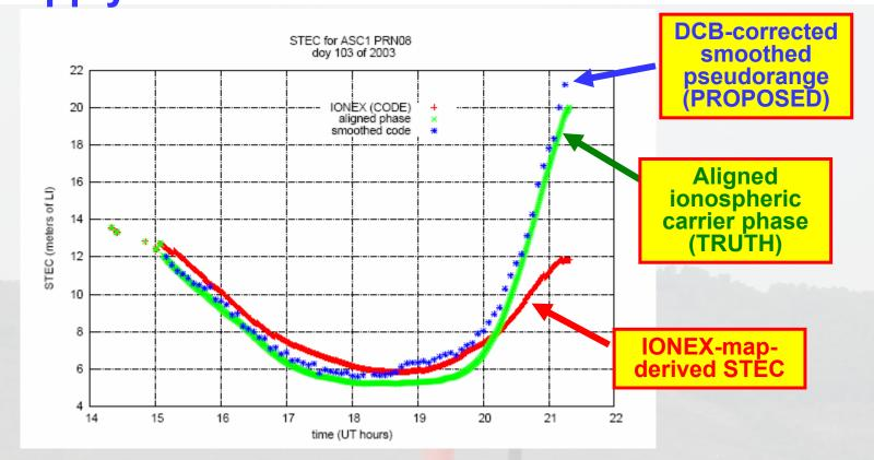
The Slant Total Electron Content, STEC, can be computed in a simple and accurate-enough way, from carrier-smoothed geometry-free combination of pseudoranges (PI≡P4), after removing previously estimated interfrequency bias values for transmitter and receiver (D, D', quite stable on time). This approach is not affected by the single-layer accuracy limitations in VTEC IONEX format, and can be understood as a new I1+I2 free carrier phase combination: Lc'=α·L1+β·L2+γ(B)·P1+δ(B)·P2+ε(B)·(D+D')
