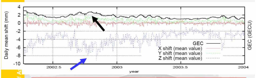
The overall I2 effect (orbit displacement + dynamical integration) produces a general averaged Z-displacement of the orbits of several millimeters.
