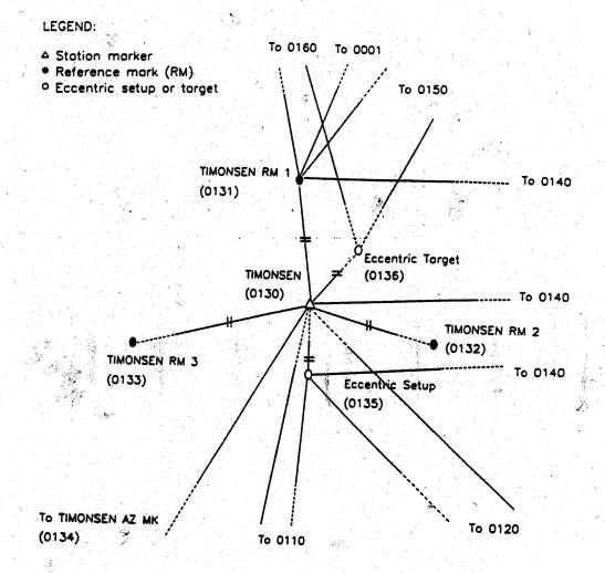
FIGURE 1-2 - STATION SERIAL NUMBERS ASSIGNED TO CONTROL POINTS AND TO PERIPHERAL POINTS.
