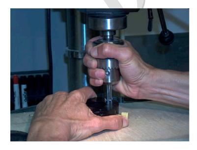
4) Using hand power only firmly hold the adapter and turn the tap in the drill press about 1/3 of a turn. Release the right hand and adjust the table up to a snug position again. Repeat until the tap bottoms out. Lower table a few inches and turn the tap back to release the adapter. Repeat for the other 2 leg holes. Cotton swabs work well to remove cuttings
