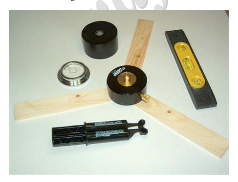
6) The use of standard wood shims under the antenna adapter will aid in leveling while the epoxy sets up. Two tubes of 1 oz. epoxy are required. After the epoxy sets, cut the wood shims away from the side of the adapter and finish the installation with a bead of caulk around the bottom edge and over the set screws to prevent moisture penetration.
