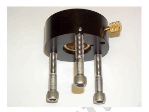
5) Insert fasteners that will hold the adapter and replace the 3 small set screws. The length should fit the installation. Shown are 3/8" – 16 stainless socket cap screws 2.5" long. A portable hammer drill with a 5/8" bit works well in drilling the holes.
