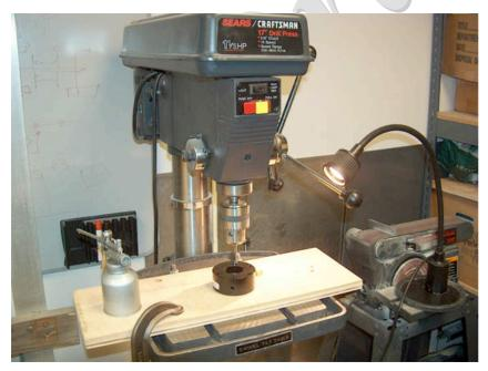
2) Remove brass center of adaptor and set up a standard drill press to cut machine threads by hand using a 3/8"- 16 Bottoming Tap similar to Greenfield #14159, or McMaster-Carr #2521A643. The drill press is an easy way to cut a straight set of threads.
