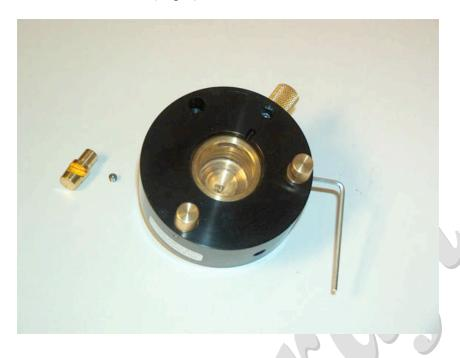
1) Remove brass legs by using a 5/64" allen wrench. Save the set screws.
