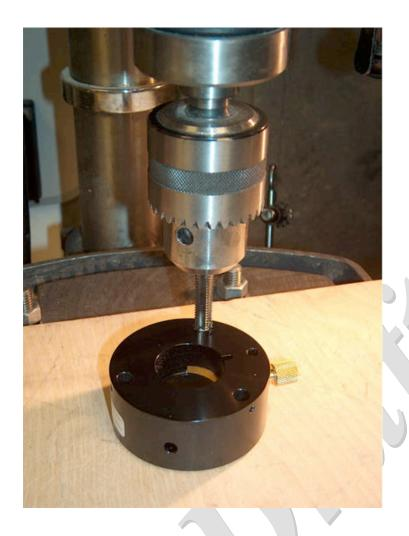
3) Unlock drill press table and adjust height to align tap with a leg hole of adapter. Snug the table up to the tap so you can start cutting threads. Apply a few drops of oil to the tap for lubrication.
