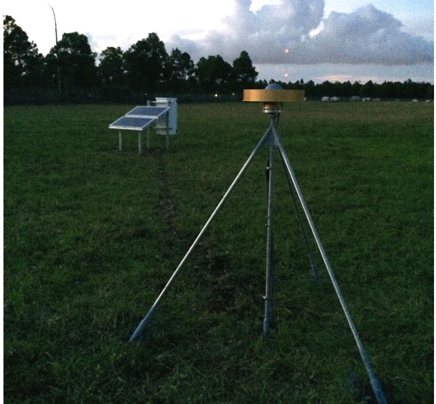
The first Foundation CORS: A Short Drilled braced monument anchored to bedrock in Richmond, Florida.
