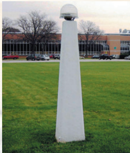
ODOT Antenna pillar/monument (CORS Classic) at Sidney, Ohio (first pillar that ODOT set)
