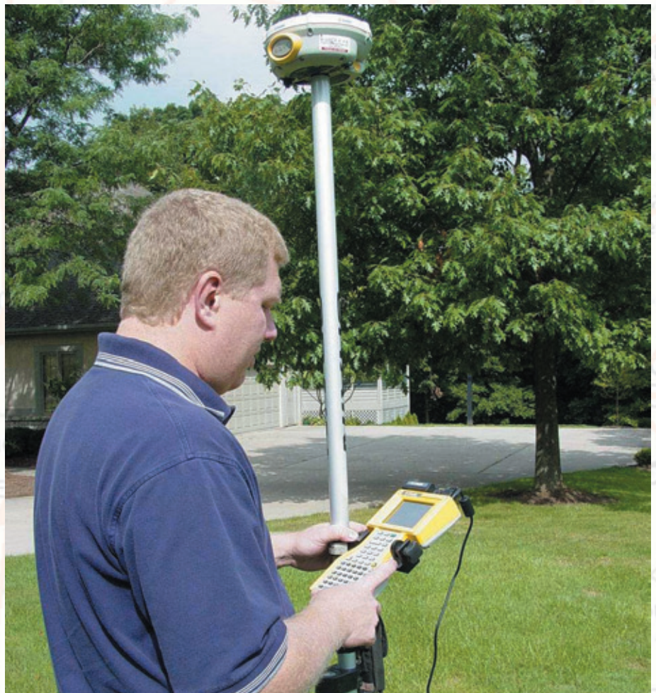
EMH&T surveyor James Pearsall, PS, collects points on the City of Granville, Ohio utilities inventory project using a single Trimble 5800 RTK GPS system with a Nextel cell phone and the ODOT VRS.
