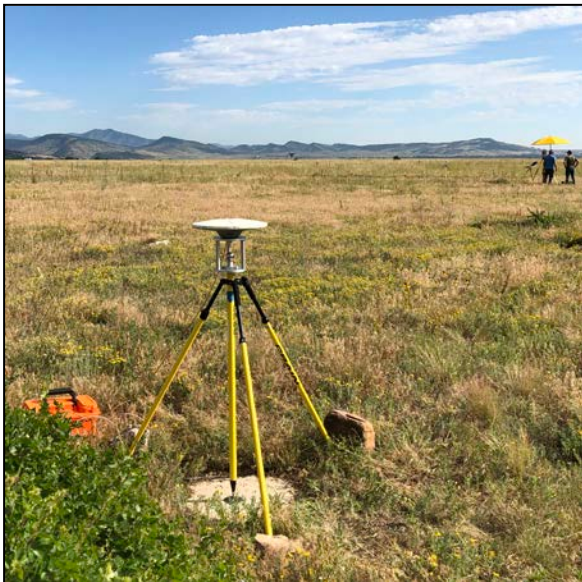
Forced-centering device to occupy a mark
