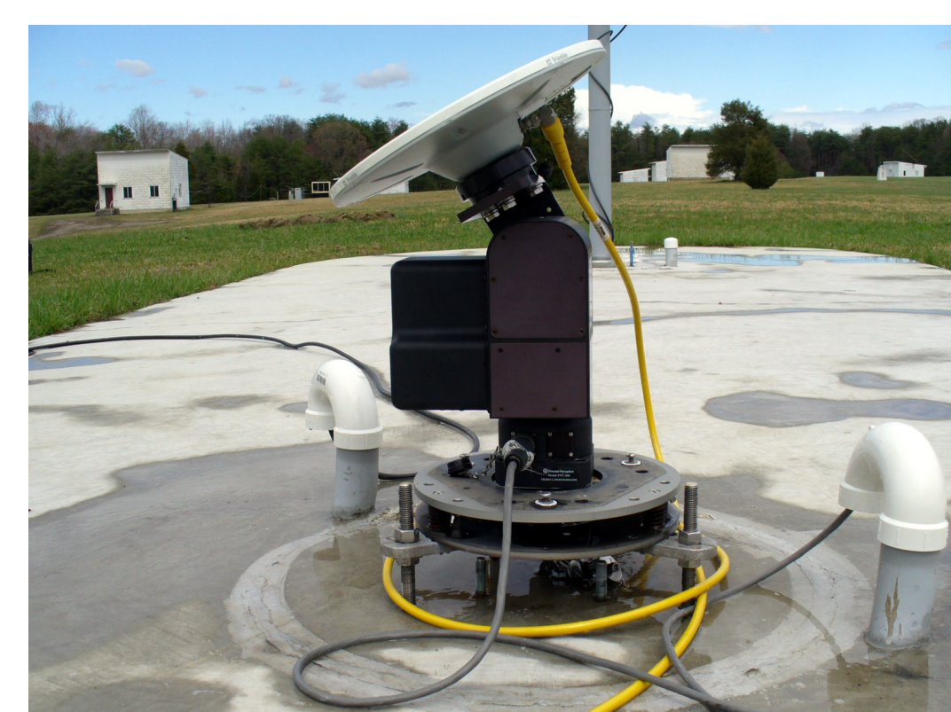
Figure 2: PTU in tilted position, with Trimble Zephyr Geodetic antenna under test.
